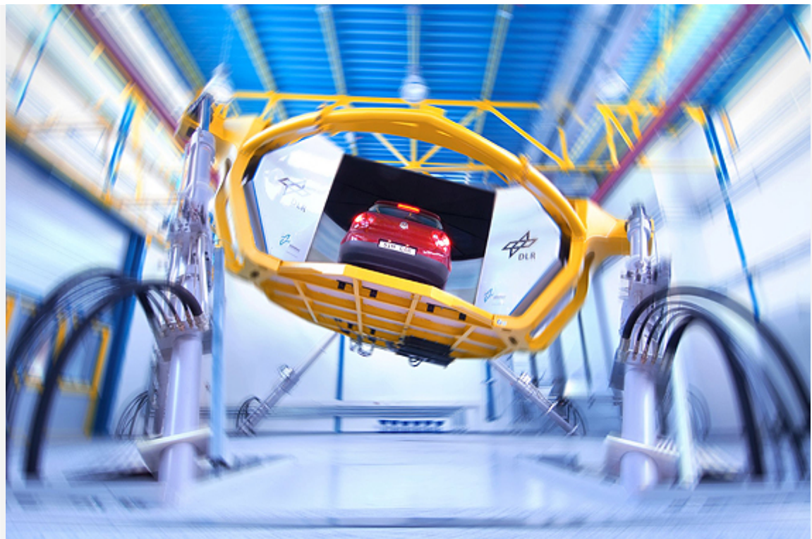
The dynamic driving simulator at the DLR Institute of Transportation Systems
