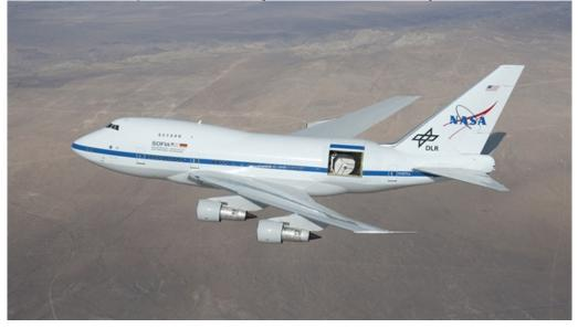
SOFIA, the Stratospheric Observatory For Infrared Astronomy, during the first test flight with the telescope door fully open, on 18 December 2009 over the Mojave Desert in California. The 2.5 metre telescope, built in Germany, is visible in the opening in the fuselage of this Boeing 747SP. The test flight with the door open helped engineers examine, for the first time under experimental conditions, the movement of air in and around the telescope and the door.
