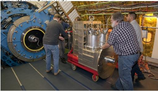
GREAT approaching the telescope. In the foreground is Steve Robinson, crew chief of SOFIA. GREAT is in fron of the telescope flange, awaiting final inspection and clearance. The pressure coupler inside the telescope tube is visible in the image.
