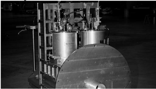
Front view of the German Receiver for Astronomy at Terahertz Frequencies, GREAT on its transport cart. The two cryostats host sensitive Hot Electron Bolometer (HEB) detectors for terahertz radiation. The operating temperature of these detectors is -269°C (4 Kelvin). The frontal plate while it was being mounted on the telescope flange (B/W image).
