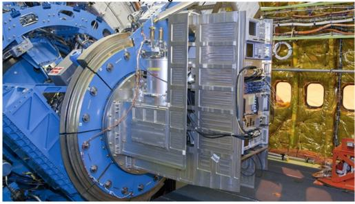
GREAT mounted on the telescope flange, which is in the nominal position (telescope at 40 degrees). During observation, GREAT will move with the telescope (+/- 20 degrees).
