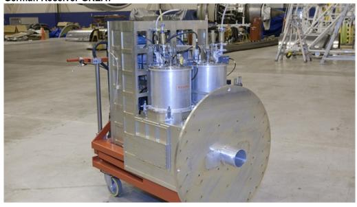
Front view of the German Receiver for Astronomy at Terahertz Frequencies, GREAT on its transport cart. The two cryostats host sensitive Hot Electron Bolometer (HEB) detectors for terahertz radiation. The operating temperature of these detectors is -269°C (4 Kelvin). The frontal plate while it was being mounted on the telescope flange.
