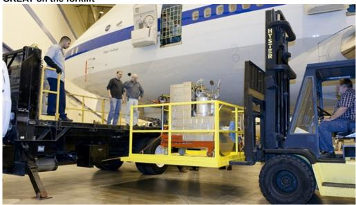
The German Receiver for Astronomy at Terahertz Frequencies, GREAT, on the forklift. Almost 700 kilograms of delicate electronics, including cart, were loaded onto the aircraft with utmost care.
