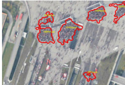
Aerial view of the entrance to the Allianz Arena in Munich: red lines mark detected groups of persons with estimated head counts.
