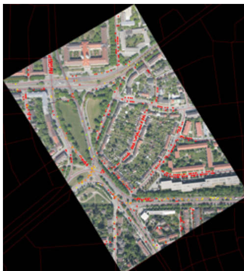
A street junction in Munich; photo taken by DLR's 3K camera system from a height of 1000 metres above ground. Coloured dots mark automatically detected vehicles and their speed. The colours represent the speed, ranging from red representing a traffic stoppage to green for fast traffic flow.
