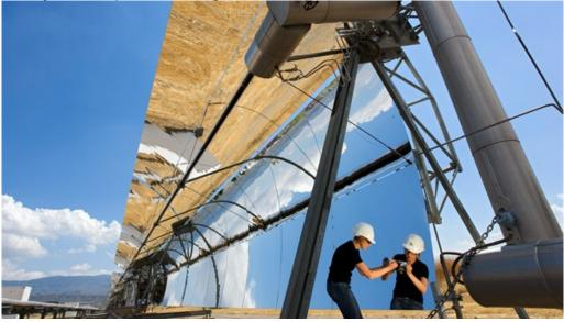
A researcher from the DLR Institute for Solar Research tests a mirror for a solar-thermal power plant. DLR has developed its own test facilities and methods for verifying quality. In important areas, they have succeeded in developing internationally recognised quality standards.
