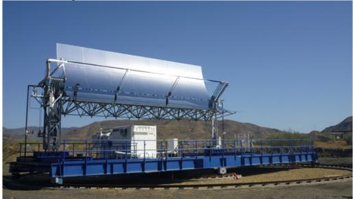
With KONTAS (Konzentrator-Teststand Almeria Spanien), energy researchers from the DLR Institute for Solar Research will be able to test parabolic trough collectors up to 20 metres long at any angle to the Sun and measure their efficiency. The new test stand can be used to evaluate complete modules of parabolic trough collectors as well as individual components such as mirrors and absorber pipes. DLR operates the new test stand at the Plataforma Solar de Almería with CIEMAT.
