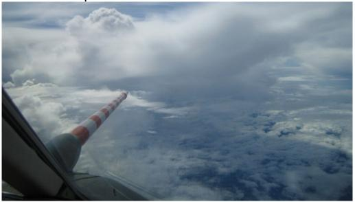
The DLR Falcon on a measurement flight. The nose boom is fitted with a five-hole sensor to measure such things as the static and dynamic pressures in the atmosphere. Through intakes on the fuselage exterior of the Falcon, scientists collected data relating to atmospheric trace gases during the SHIVA flights, which enabled them to demonstrate that biogenic halogen compounds can be transported into the higher layers of the atmosphere by tropical storms.
