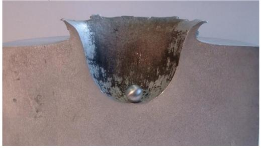
In a laboratory experiment conducted at the European Space Agency (ESA), a small aluminium sphere was fired at an 18-centimetre-thick aluminium block. The projectile was travelling at about 6.8 kilometres per second. The image clearly depicts the resulting damage. An active satellite would experience similar effects in the event of a collision with space debris.
