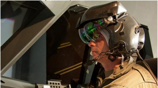
A test candidate from the Germany Armed Forces during the first trial of the new helmet mounted display in the generic cockpit simulator at the DLR Institute of Flight Guidance.
