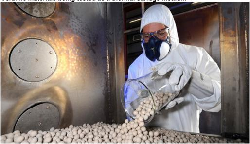
Researchers at the DLR Institute of Technical Thermodynamics are testing ceramic materials (pictured here), molten salts, concrete and natural stone for use as thermal storage media.
