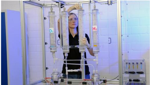
Electrolysis test stand with DLR-developed electrodes for alkaline water electrolysis. DLR researchers are working on more efficient methods of producing hydrogen by electrolysis.
