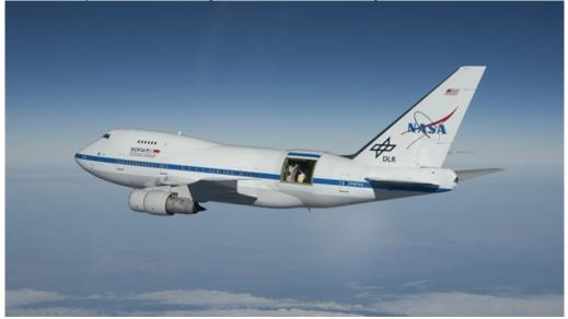
The Stratospheric Observatory For Infrared Astronomy, SOFIA, during its first test flight with its telescope exposed, on 13 July 2010. The German-built 2.5-metre infrared telescope is visible through the opening in the aircraft.
