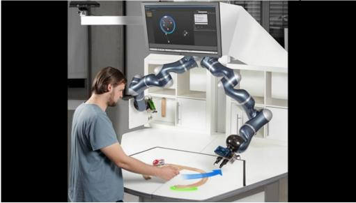
The RMC has introduced a paradigm shift in the area of safe, intuitive collaboration between humans and robots; the new generation of robotic assistants puts the human at the core of the robotic system. The two-armed 'co-worker' automatically adjusts its activity and the level of safety to suit the distance from its human colleague. This means that the human can interactively and very easily reprogram the robotic software at any time – just by moving.
