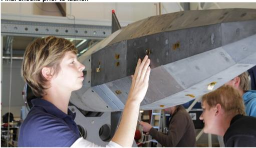
DLR researcher Hannah Böhrk examines the porous thermal shield tiles, through which nitrogen flows during flight. The gas creates a film over the SHEFEX II craft and performs active cooling during re-entry.
