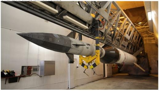
SHEFEX II and its launch vehicle still in the horizontal position; just before lift-off, the roof opens and the launch tower is raised to the vertical position.
