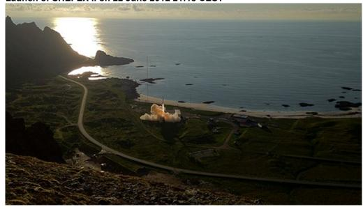
After a 10-minute flight, the sharp-edged SHEFEX II spacecraft landed safely west of Spitsbergen. DLR researchers launched the seven-ton and roughly 13-metre-long rocket and its payload from the Andøya Rocket Range in Norway at 21:18 CEST on 22 June 2012. As it reentered the atmosphere, SHEFEX withstood temperatures exceeding 2500 degrees Celsius and sent measurement data from more than 300 sensors to a ground station.
