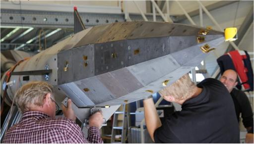
A few days before the launch, DLR researchers assemble the various components of the SHEFEX II vehicle. The spacecraft is notable for its sharp-edged design.
