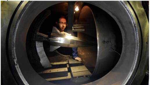
Technician Mario Jünemann prepares the SHEFEX II model for its test in the high-enthalpy wind tunnel at Göttingen. This involves incorporating 50 pressure sensors and 60 thermocouple elements to the projectile. During this test, thousands of data values are recorded within a thousandth of a second.
