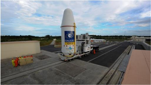
The 'upper composite' of the launch system, made up of the launcher's fourth stage, Fregat-MT, the two Galileo satellites and the fairing.
