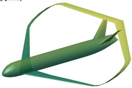
In the futuristic 'box wing' geometry, two wings unite above the fuselage.
