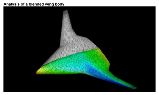
Aerodynamic analysis of a blended wing body; the colours indicate the pressure distribution.
