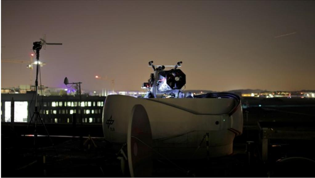
The quantum key transmission experiment took place in Oberpfaffenhofen, using the optical ground station at the DLR Institute of Communications and Navigation and the Dornier Do 228-212 research aircraft. The laser beam sent from the aircraft was received by the ground station, recorded with specially developed measuring equipment and analysed.
