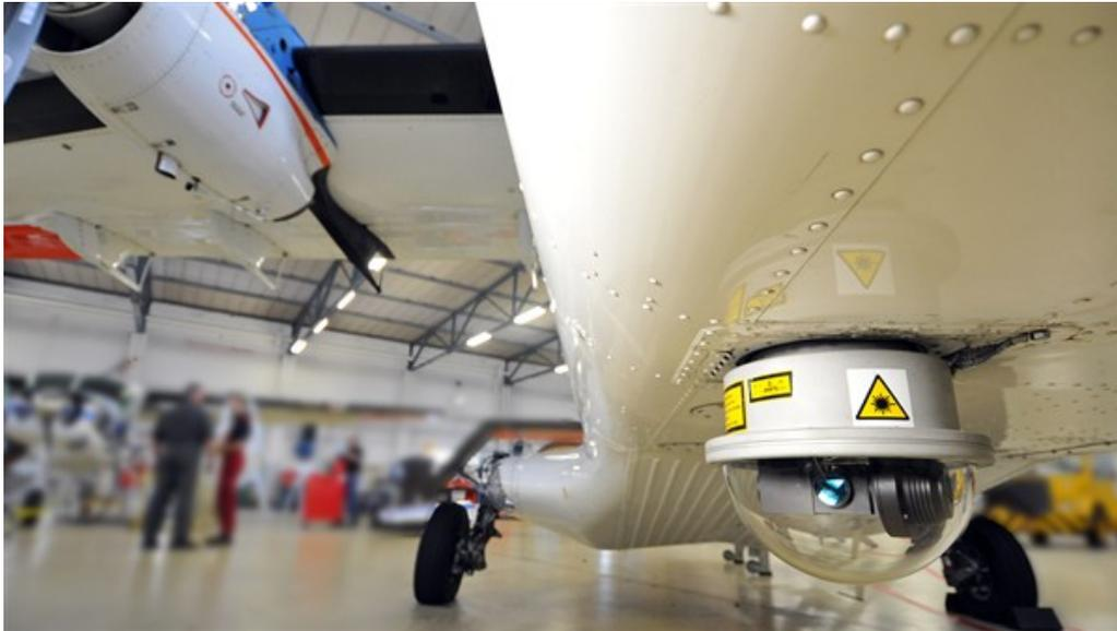
The external part of the laser terminal is attached to the fuselage of the DLR Do 228-212 research aircraft.
