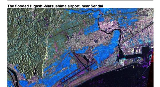
This radar image, acquired by the German Earth observation satellite TerraSAR-X on 12 March 2011 at 21:43 CET, shows the impact of the tsunami on Higashi-Matsushima Airport and the port of Ishinomaki, near Sendai, on the east coast of Japan. The blue areas indicate the flooding; the magenta-coloured areas show the extent of the destroyed infrastructure.
