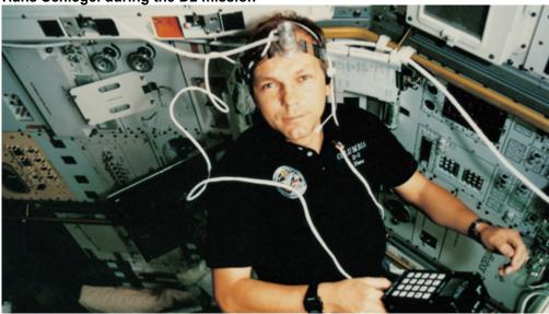
Astronaut Hans Schlegel in the Spacelab wearing an ultrasonic measurement device on his forehead. Under the AR-TISSU experiment, tissue thickness and stability along the axis of the body were studied under microgravity conditions. The picture was taken during the 1993 D2 mission.
