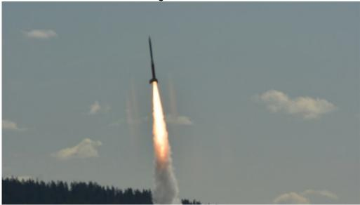
Close to four minutes of microgravity prevailed in the sounding rocket MAPHEUS-4, which was launched on 15 July 2013 at 07:53 local time, from the Esrange Space Center in northern Sweden. During the four minutes of microgravity, researchers from the DLR Institute of Materials Physics conducted various experiments.
