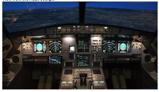
Cockpit of the A320 simulator. At the left centre of the image is the display of the recently tested pilot assistance system.
