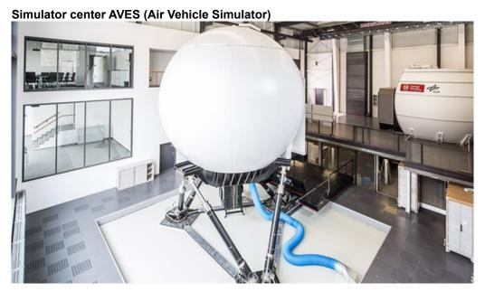
The simulation center is home to a moving and a stationary simulator with an interchangeable cockpit.
