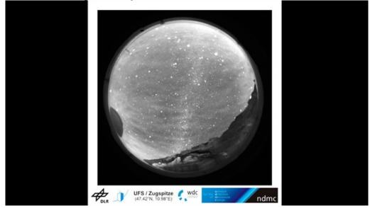
At the research station Schneefernerhaus the scientists are able to observe gravitiy waves in the airglow at night. In this picture the wave signatures are clearly visible in the horizontal line. The picture was taken on 8 October 2013 with the All-Sky Airglow Imager BAIER.
