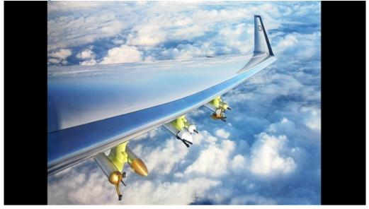
HALO carries one of the world's most modern sets of cloud research instrumentation. The 'underwing stations' carry the PMS probes – particle measurement instruments for sampling cloud droplets and ice crystals.
