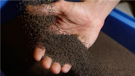
Ceramic particles about one millimetre across are directly irradiated in the receiver – they act as both heat exchangers and a storage medium.
