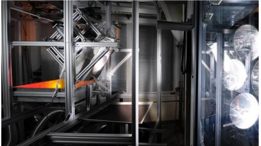
Novel receiver being tested with high-performance radiators at the DLR solar furnace in Cologne.
