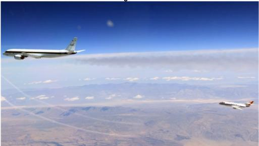
Behind the DC-8, the scientists on board the DLR Falcon measured the exhaust gas composition.
