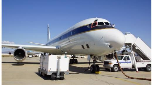
During the research flights, the four CFM56 engines of the DC-8 alternated between regular JP-8 jet fuel and a one-to-one mixture of JP-8 and the biofuel HEFA (Hydroprocessed Esters and Fatty Acids). HEFA is obtained from the oil of Camelina plants.
