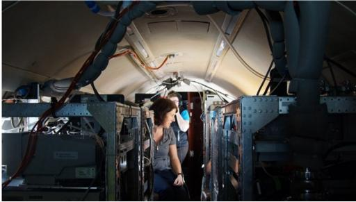
DLR researchers focus on measurements of the biofuel exhaust emissions of soot and sulphur particles, as well as the size and shape of the ice crystals in the condensation trails.
