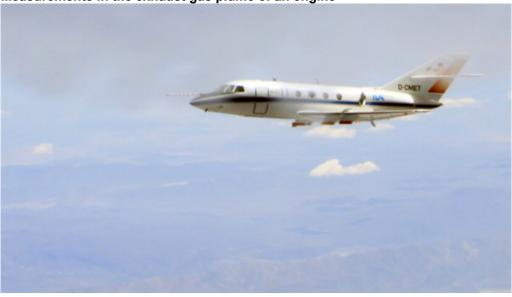
The DLR Falcon flies with its measuring inlets in the upper part of an engine exhaust gas plume. Credit: NASA.
