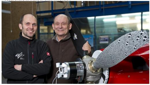
Fritz Boden and Boleslaw Stasicki from the DLR Institute of Aerodynamics and Flow Technology in front of their invention – a rotating camera mounted in the hub of a propeller. They have used this to make the deformation of a propeller blade during flight visible for the first time.
