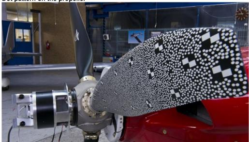
Not just the camera and its housing have been developed by the DLR researchers in Göttingen – so too has the measurement technology employed. This involves using two cameras with different angles of view (stereoscopy) to take images of the object under investigation. A computer identifies the equivalent points in the images – the dot pattern helps with this. Knowing the position and attitude of the cameras enables the entire surface being observed to be represented in 3D.
