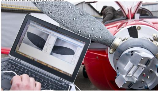
The camera is aligned with the propeller blade and rotates in synchrony with it. The images are transferred to a computer via a wireless network.
