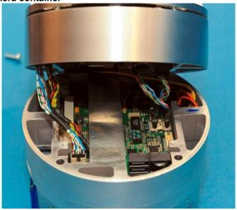
The researchers from Göttingen placed the camera, a miniaturised computer and other electronics inside a metal container that protects them from the extreme loads exerted by the rotating propeller.
