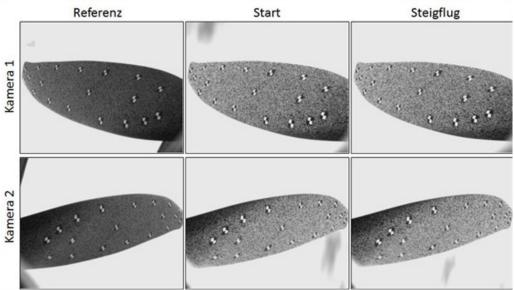
Sequence of images from both cameras. The propeller blade is seen from various viewing angles and in different flight situations.
