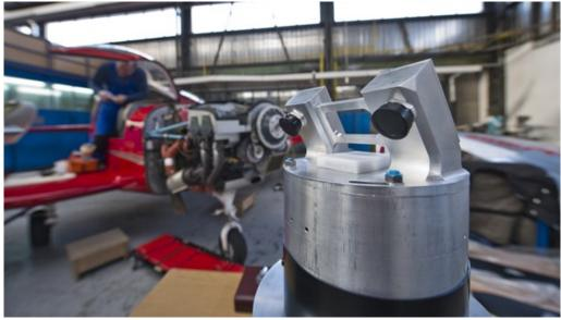
The researchers from Göttingen placed the camera, a miniaturised computer and other electronics inside a metal container that protects them from the extreme loads exerted by the rotating propeller.
