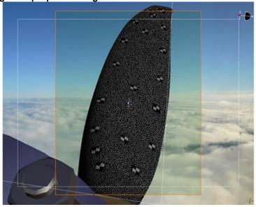
Photomontage from a recording of a propeller blade in flight against a background of clouds.
