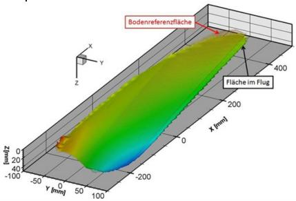
Computer representation of the surface of the propeller calculated during flight. A deflection can be seen in flight (Fläche im Flug) compared to the shape on the ground (Bodenreferenzfläche).
