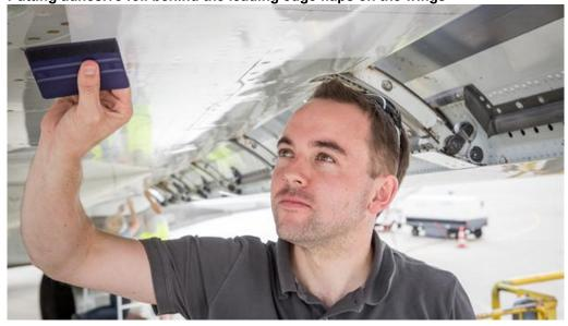
Over the course of the flight tests, researcher Gloß collects insect contamination on adhesive foil stuck behind the leading edge flaps on the wings. The foils are taken directly to the laboratory at the end of the day's flights, where they are digitised using a scanner.
