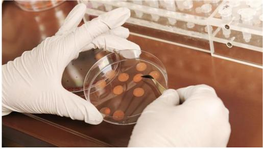
The specimens being prepared for the BIOMEX and BOSS experiments in the German Aerospace Center (DLR) laboratory. The organisms will be placed in a space environment in the EXPOSE-R2 system fitted to the exterior of the International Space Station.
