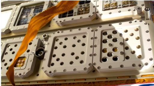
BIOMEX will be installed in the EXPOSE-R2 system
