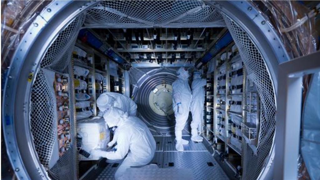
6555 kilograms of cargo were stowed on board the European space transporter ATV-5 'Georges Lemaître'. This included food for the astronauts, supplies of fuel, water and air, and scientific experiments. On 30 July 2014, the Automated Transfer Vehicle lifted off en route to the International Space Station.
