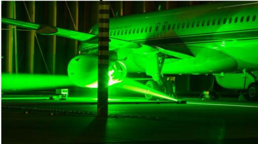
To visualise the turbulent speed and density fluctuations, the scientists used optical measurement systems that work with special cameras and lasers and are synchronised with an array of microphones.
