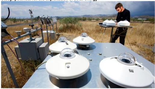
A DLR scientist uses a rotating shadowband irradiometer to measure the direct solar radiation.
