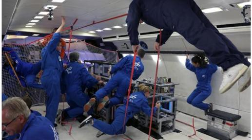
The TEMPUS facility is used on DLR parabolic flights to melt and resolidify samples in weightlessness. The data is aimed at enabling casting processes on Earth to be carried out more effectively in future.
