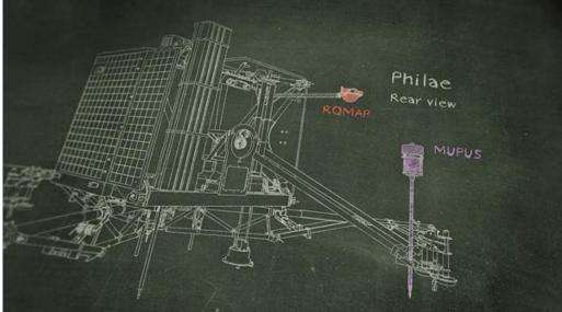
The thermal probe MUPUS measures the temperature on and beneath the comet's surface, as well as the thermal conductivity of the surface material.
