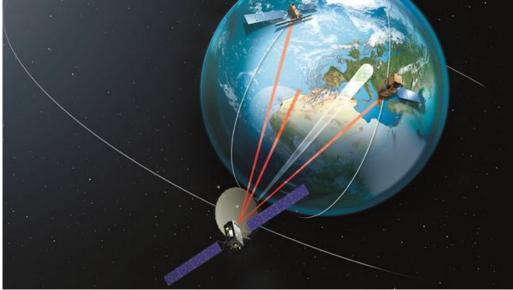
EDRS is an ESA programme for an independent European satellite data relay system. It is designed to significantly reduce the time delay in the transmission of large amounts of data.
