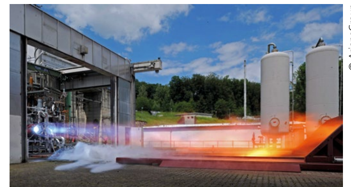
Test of a combustion chamber on the P3 test rig
