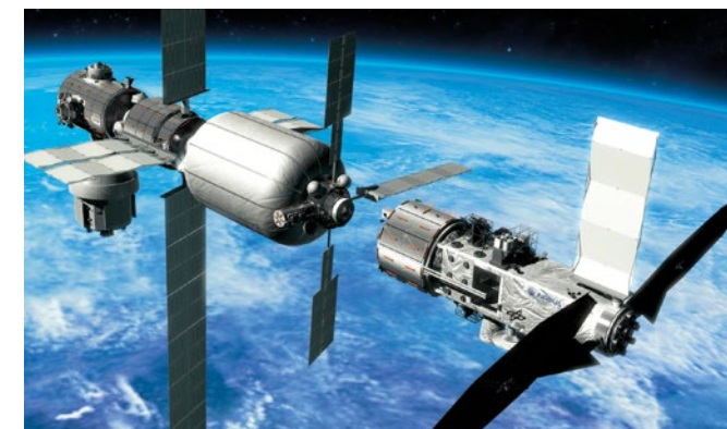
The modular Orbital Hub with the base platform and the free flyer
