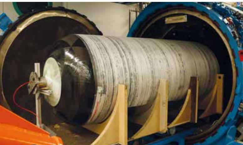
Ultralight CFRP high-pressure tank for hydrogen
