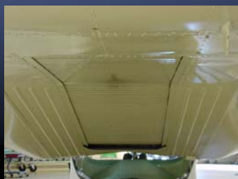
2 large openings in the bottom of fuselage with rollerdoor cover 2060 mm x 515 mm Ø 500 mm
