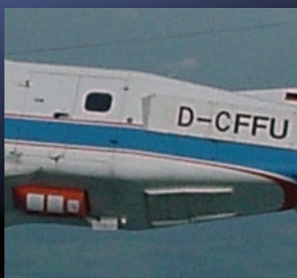
2 large openings in the bottom of fuselage with rollerdoor cover 2060 mm x 515 mm Ø 500 mm
