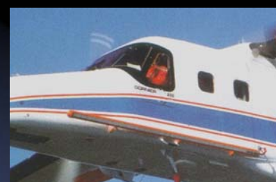
hardpoints at side of fuselage for up to 50 kg
