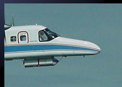
hardpoints under the fuselage for up to 200 kg
