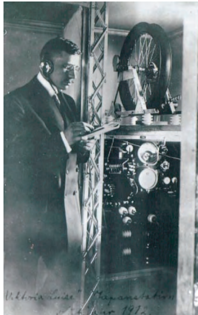
Figure 1-2: Dr. Max Dieckmann and the wireless radio station on-board the airship "Victoria Luise", 1912.
