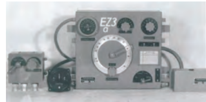
Figure 1-9: Specialised airborne receiver for direction and route finding.
