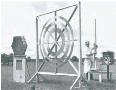
Figure 1-12: An engineer during experiments with wave guide and Fresnel lens antennas.
