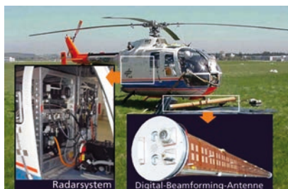
Digital beamforming demonstrator on a DLR helicopter
