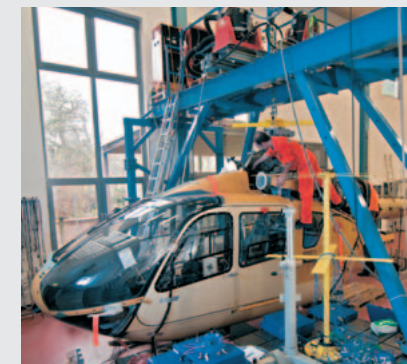
Mid-air rotor blade vibrations are simulated on an EC135 helicopter, with the test assembly affixed to the rotor head.
