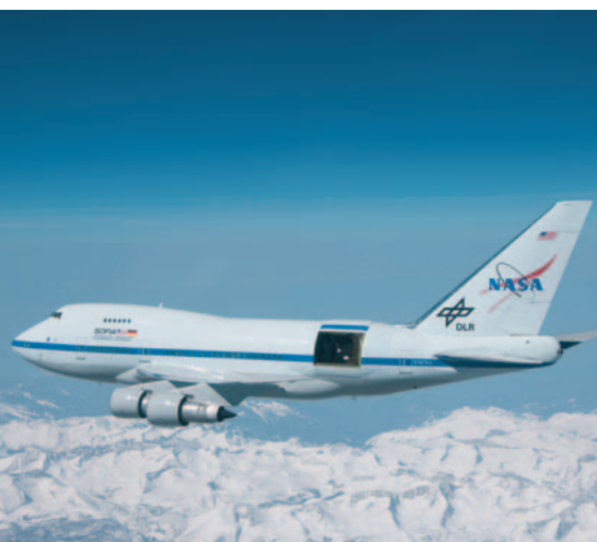
SOFIA on a test flight in December 2009. The Boeing 747SP, which has a shorter fuselage than a standard 747, spent years undergoing modifications.
