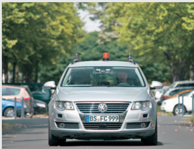
The DLR test vehicle FASCar receives information from the next set of traffic lights about how long its current red phase will last
