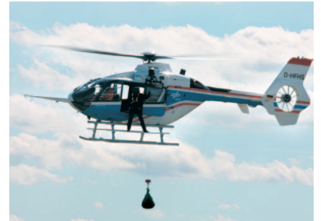
During flight tests with DLR's research helicopter (FHS), its rescue hoist was examined, among other things.
