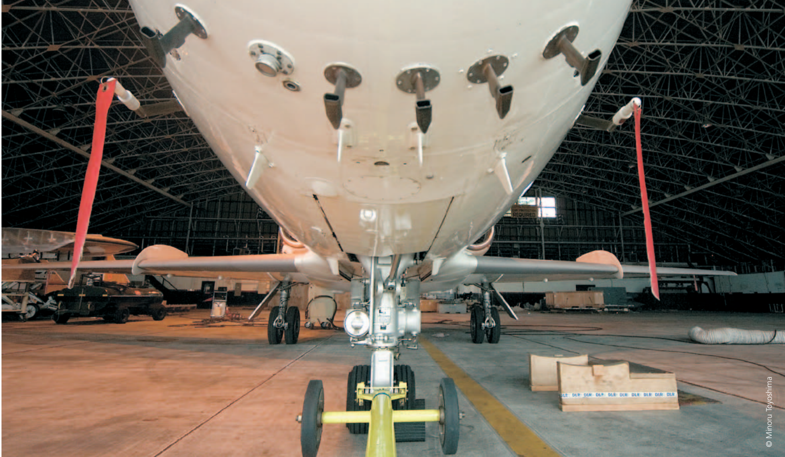
The measurement aircraft has heated inlets near its nose, through which ambient air is fed to temperature and humidity sensors during flight.
