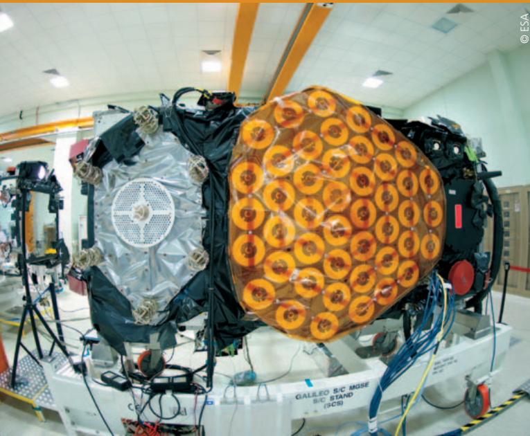
Galileo satellite number one during mechanical testing at Thales Alenia Space in Rome during May 2011
