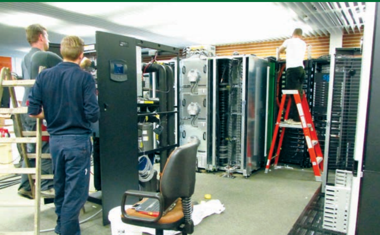
The high-performance computer, which was inaugurated in October 2013, is smaller than its predecessor, yet significantly faster; the new C 2 A 2 S 2 E cluster can perform up to 262,000,000,000,000 floating point operations per second.
