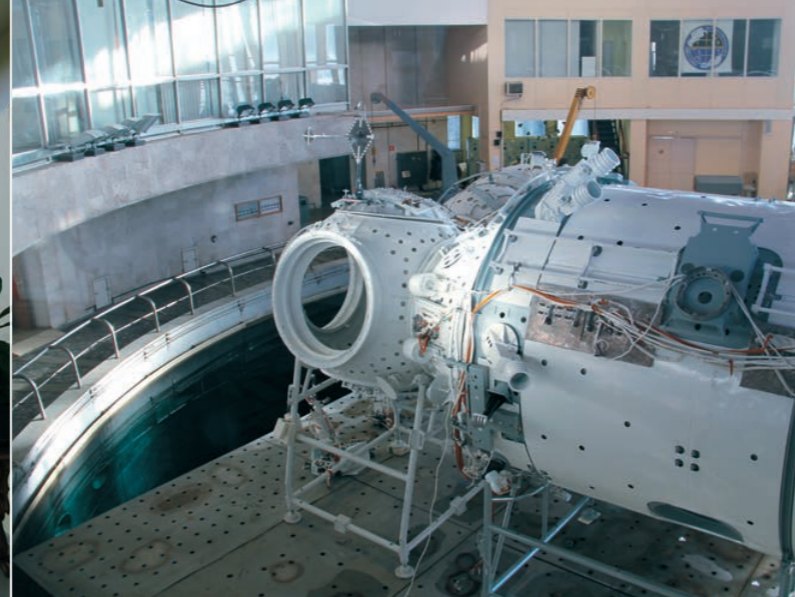
Underwater training for the extra-vehicular activity: as soon as the modules are lowered into the water, the astronauts can start training almost as if in the weightlessness of space.
