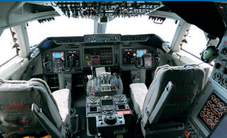
A converted Boeing 747SP carries the infrared observatory to an altitude of around 42,000 feet. The avionics in the aircraft cockpit were modernised in 2012. Modern, digital displays were installed to replace the previous analogue instruments.
