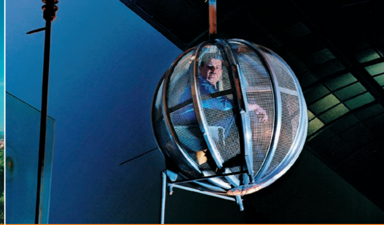
220,000 volts and very noisy – high voltage current test using the Faraday Cage.
