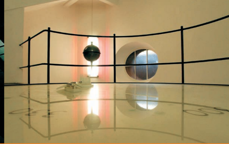
Fascinating presentation – the Foucault Pendulum demonstrates the rotation of the Earth.
