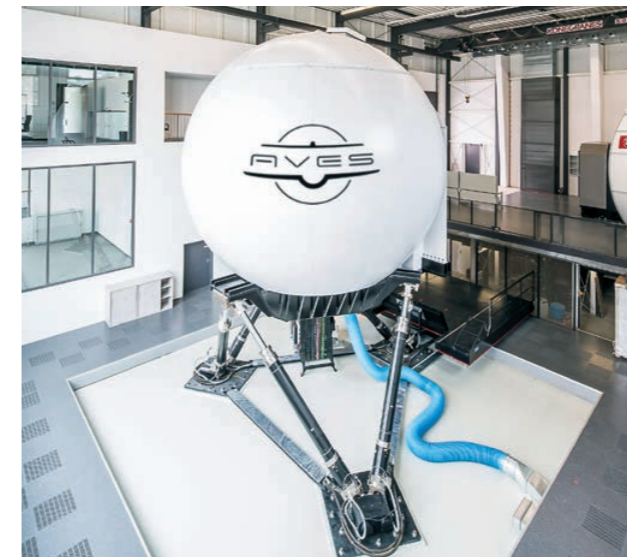
The eye-catching AVES full flight simulator in the hall at the simulator centre. The rounded structure, which is attached to a movable platform, can be used for both airliner and helicopter cockpits.
