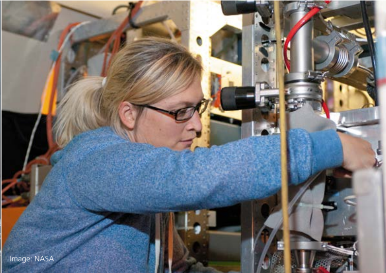
Anke Roiger prepares a mass spectrometer for measuring sulphur gases by flushing it with high purity nitrogen
