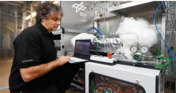
The hydrogen tank is filled with solid materials that absorb the gas like a sponge and improve the performance of the tank.
