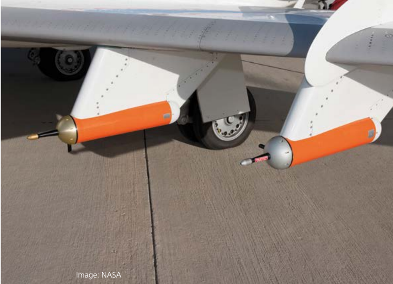
Particle measurement probes under one of the DLR Falcon’s wings
