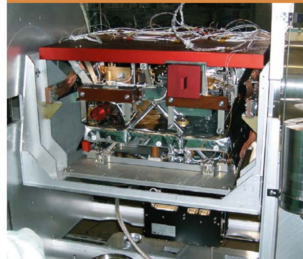
The VIRTIS spectrometer on the Rosetta spacecraft has already delivered its first data
