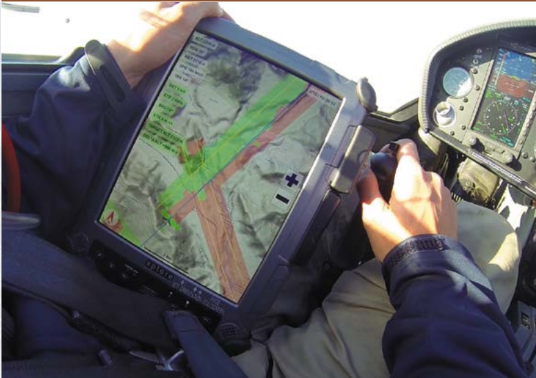
The flight guidance system assists the pilots during the systematic flight pattern. The green areas were flown over and the expected large brightness differences encountered.
