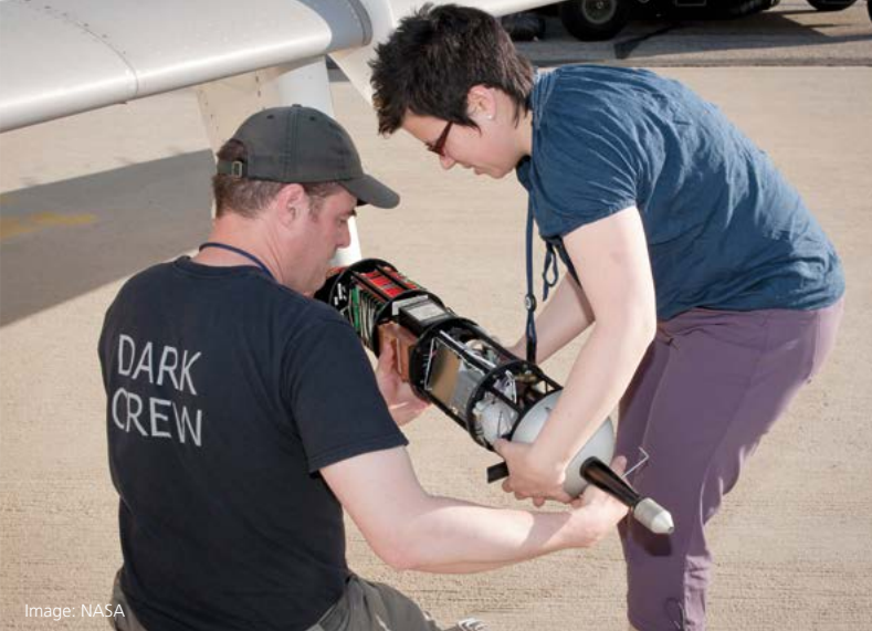
Daniel Sauer and Bernadett Weinzierl install a soot measurement probe in the instrument holder
