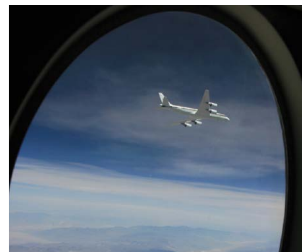
The DC-8, seen from the window of the DLR Falcon, shortly before the Falcon is positioned behind it to measure the exhaust gas plume.
