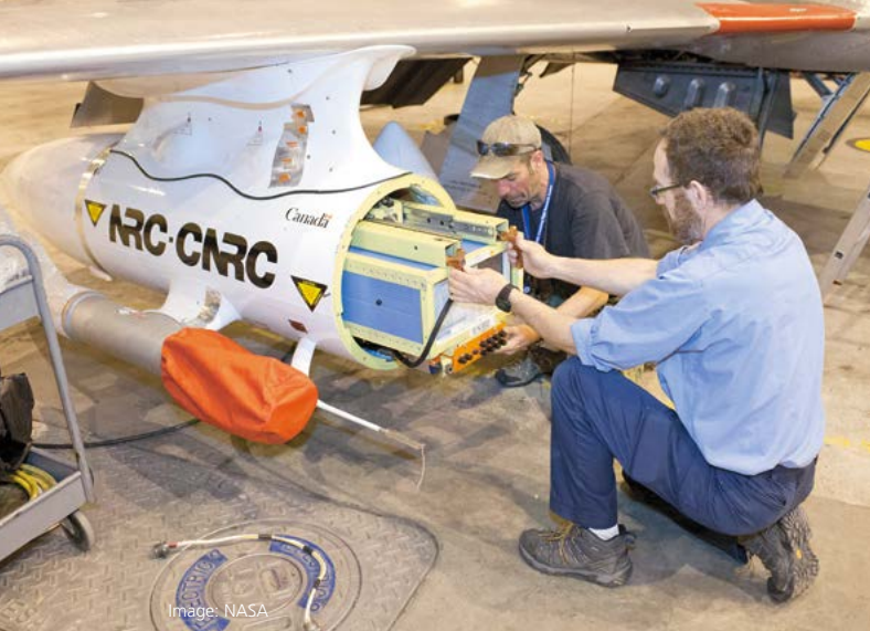
The sensor for measuring wake turbulence is installed in an underwing pod the Canadian T-33 research aircraft
