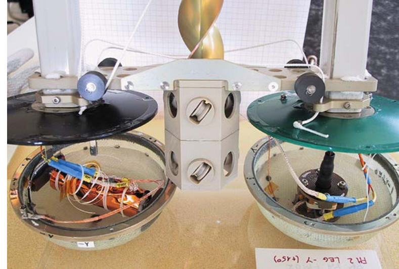
The SESAME instrument sensors are mounted on the feet of the lander, and will use electrical and acoustic methods to examine the composition of the cometary surface.
