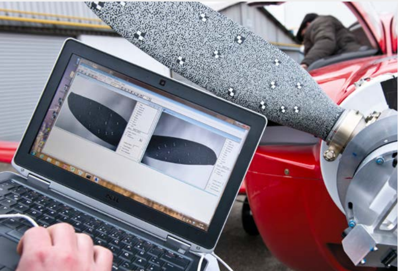
Two cameras film the propeller blades from different angles. The equivalent points are identified by computer with the help of the attached dot pattern. Having knowledge of the position and orientation of the cameras, the entire surface of the propeller can be visualised in three dimensions.
