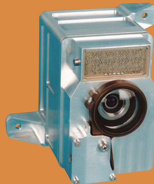
The ROLIS camera on the bottom side of Philae will acquire its first images during the landing on 67P/Churyumov-Gerasimenko
