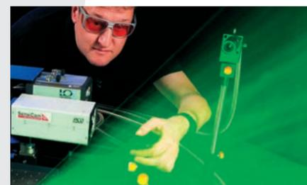
The measurement technology in a laboratory setting: A crystal fibre introduces a laser beam into the exhaust plane of the combustion chamber. An image guide is then used to observe the scattered light as if through a keyhole.
