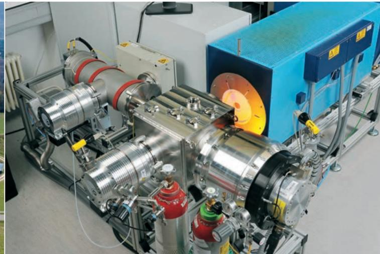
DLR high-temperature flow reactor, consisting of a high-temperature furnace (blue housing) and the molecular beam mass spectrometer
