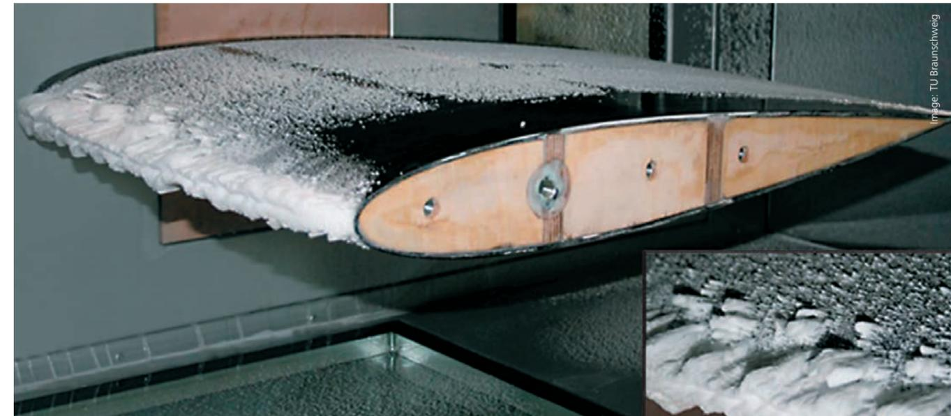
Analysing the phenomenon of large supercooled droplets on aircraft wings in the ice wind tunnel at TU Braunschweig
