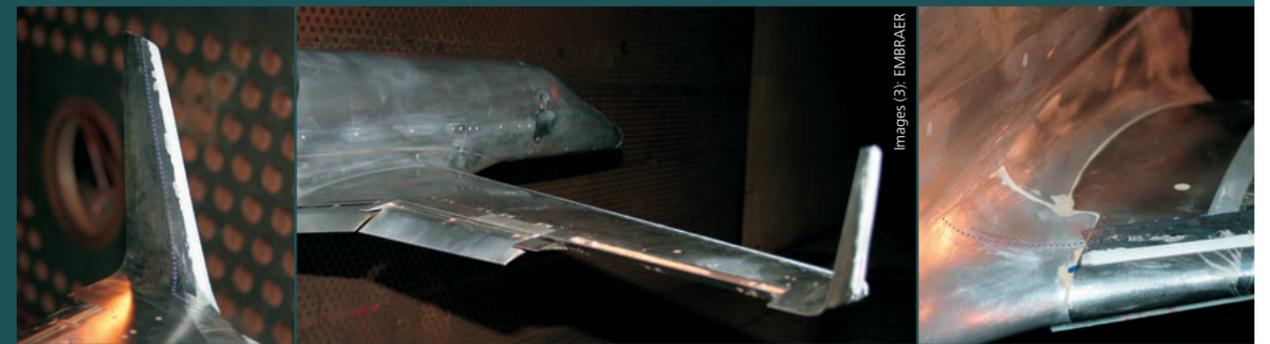
Phenom 300 wind tunnel tests with artificial ice shapes in the Russian Central AeroHydrodynamic Institute TsAGI
