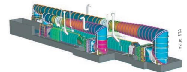
Graphical representation of the Vienna Climatic Wind Tunnel – a state-of-the-art wind tunnel built in accordance with the old Göttingen design.
