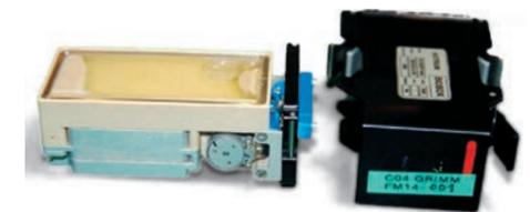
On the ISS, the cell cultures prepared by scientists from the University of Magdeburg were subjected to microgravity conditions. Their 'habitat' was the CellBox experiment chamber, which is roughly the size of a smartphone. The image shows the chamber, equipped with a pump and tanks for supplying nutrients and fixing the cells. After 30 days in space, the cell cultures and the small experiment chambers were returned to Earth in the Dragon capsule, where they were analysed by the scientists.
