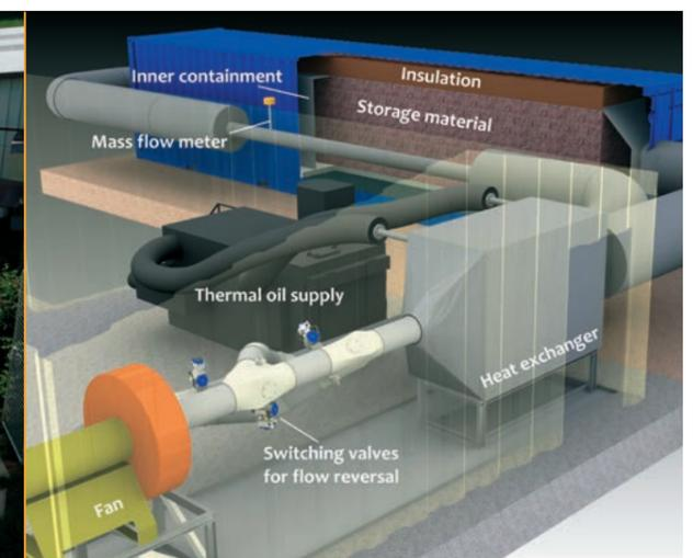
The CellFlux concept for heat transfer and storage
