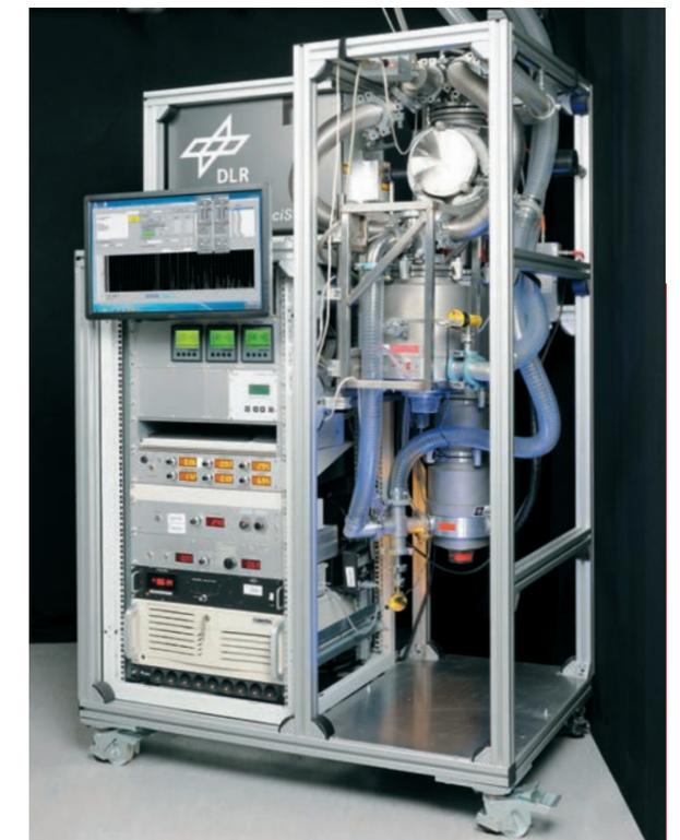
The mobile mass spectrometer – developed by DLR for exhaust measurements and analysis of both gases and nanoparticles.
