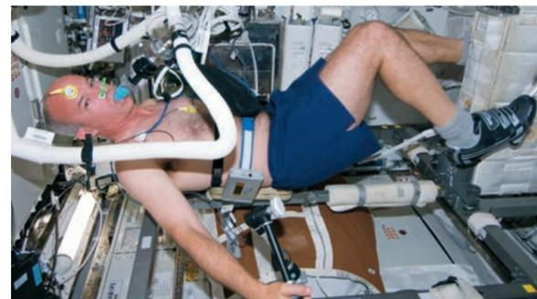
Thermal experiment being conducted on board the ISS in 2009 – two sensors attached to the skin (yellow patches on the head and chest) provided continuous measurements of core body temperature as the US NASA astronaut Jeffrey Williams completed a physiological performance test.
