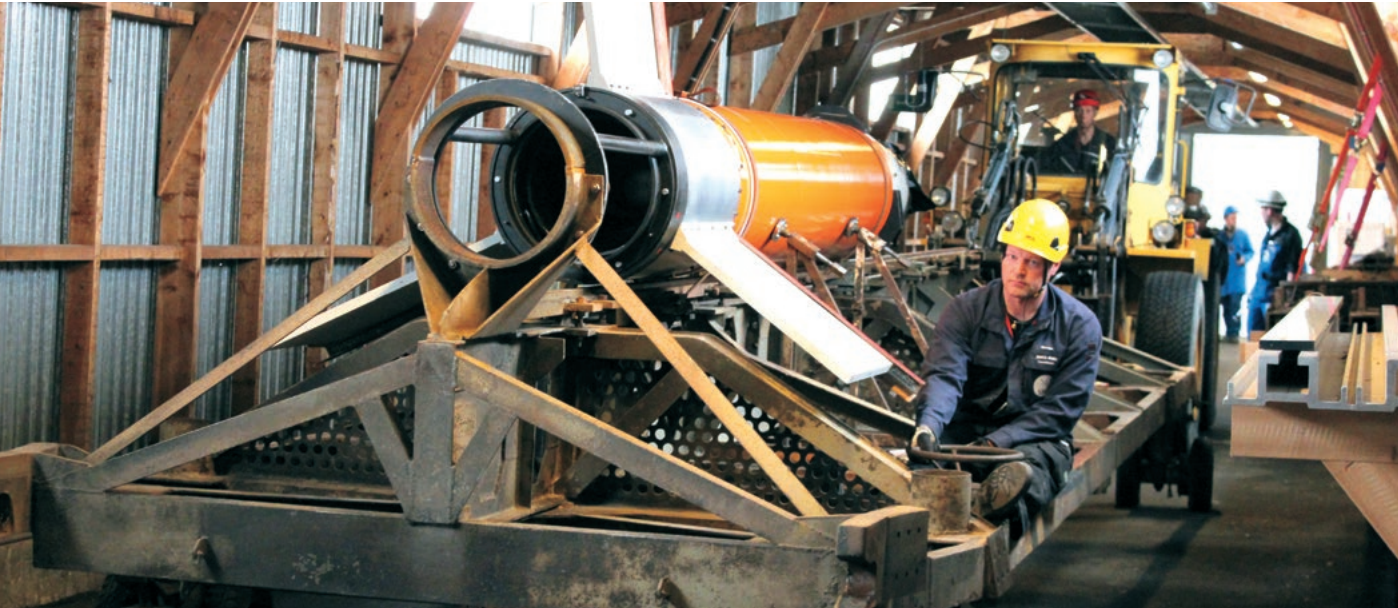
The Brazilian-developed nozzle, ready for assembly.
