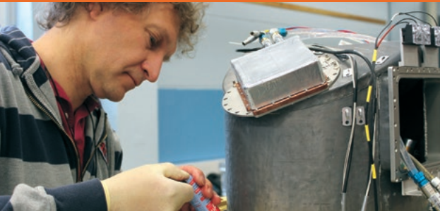
X-RISE: X-ray system designed to record diffusion and solidification processes with a camera during every second of the flight into microgravity.
