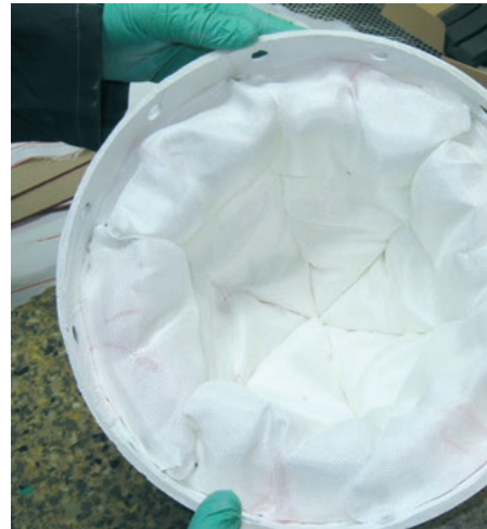
The finished WHIPOX™ half-shell, lined with the insulating pillows.
