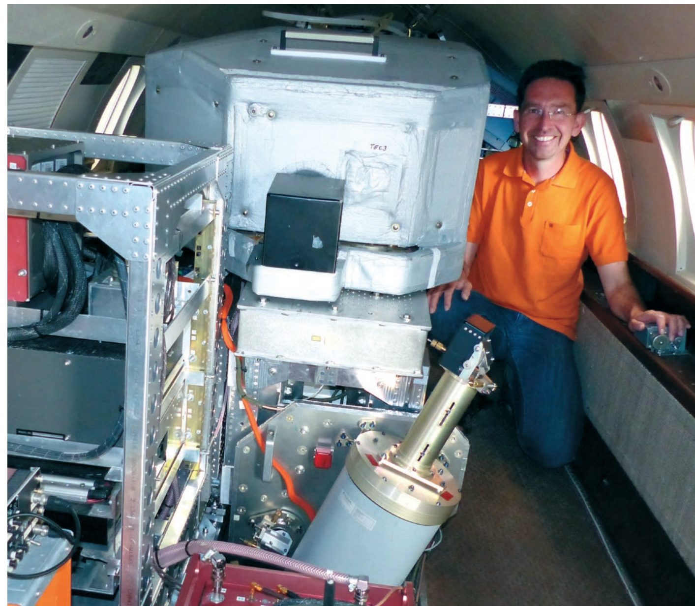
Inside the cabin of the DLR Falcon. Here, DLR scientist Oliver Reitebuch of the Institute of Atmospheric Physics with the two wind lidar instruments. The optical receiver of the satellite prototype ALADIN is well insulated for thermal stabilisation (grey box, image centre).
