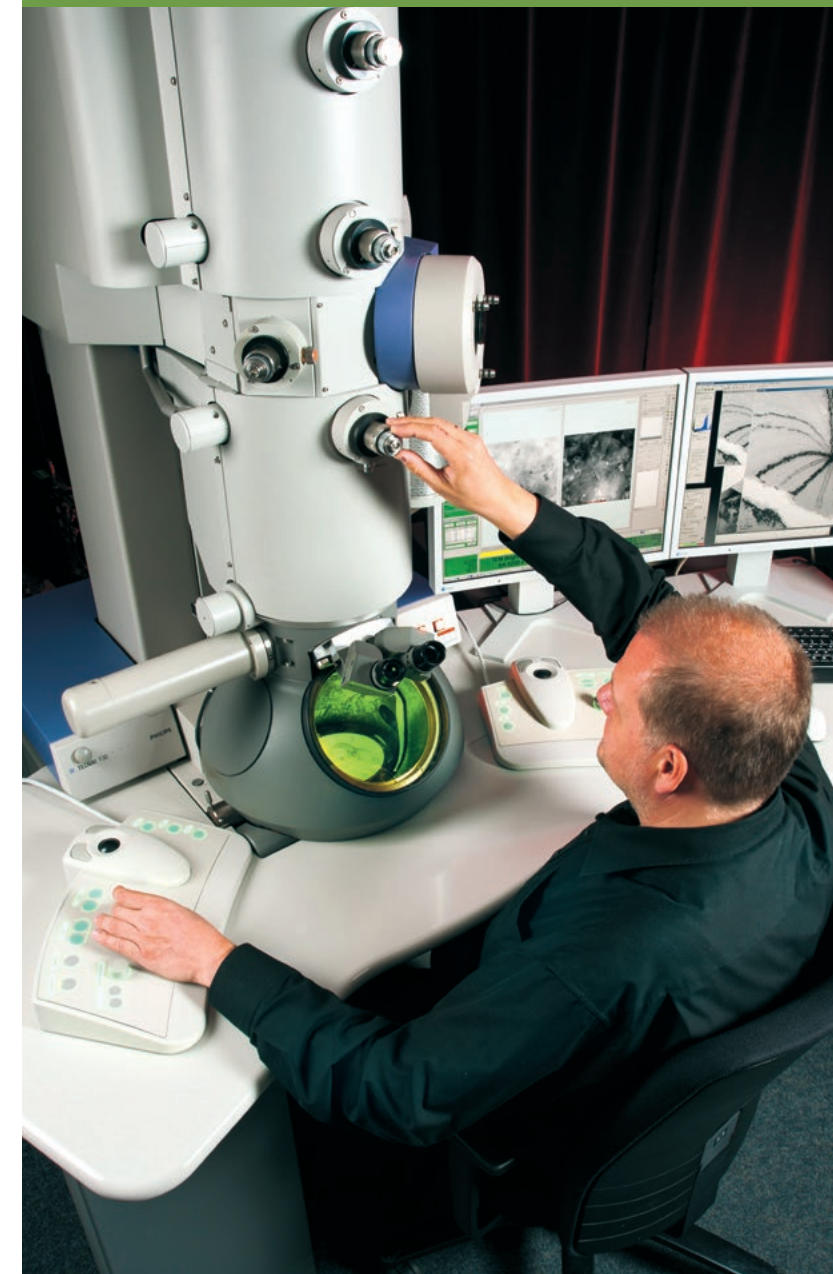
Klemens Kelm operating a Philips Tecnai F30 transmission electron microscope. This instrument is used at the DLR Institute for Materials Research to investigate new materials, such as titanium aluminide alloys, which are used in turbine engines.
