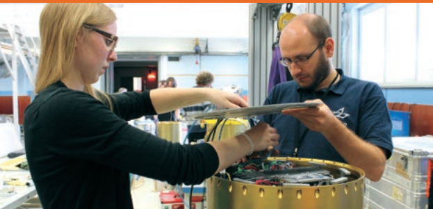
GOLD-ESL: In the electrostatic levitator, samples will be melted while floating without coming into contact with the wall of the crucible.
