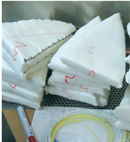
Small insulating pillows protected the electronics from the heat
