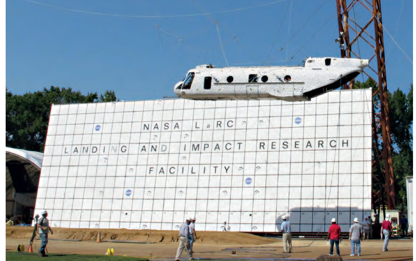
With the help of high-speed cameras each of the more than 8000 black dots painted on the helicopter skin could be tracked and the deformation of the fuselage analysed
