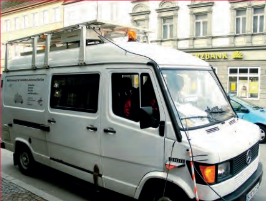
In 2002, DLR researchers investigated the radio channel between a measurement bus and a Zeppelin using the Channel Sounder.
