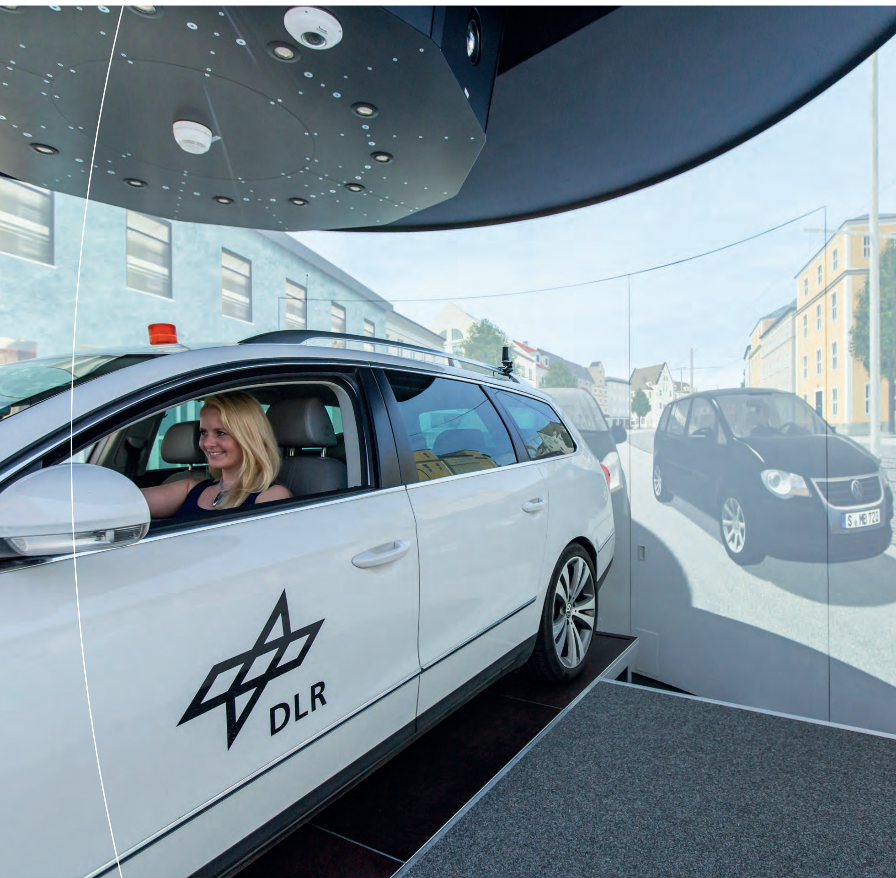
Driving simulation using DLR's Virtual Reality Laboratory: A 360-degree representation of the surroundings conveys a realistic driving experience.
