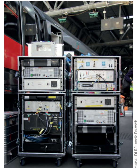
The Channel Sounder consists of a transmitter and a receiver unit. The receiver reveals how the radio signal is reflected by the environment.
