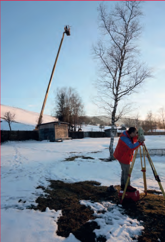
To measure the ground reflections of a radio signal emitted from an aircraft or a satellite, the scientists installed the Channel Sounder on a 40-metre-high crane during tests in 2014 and 2015.
