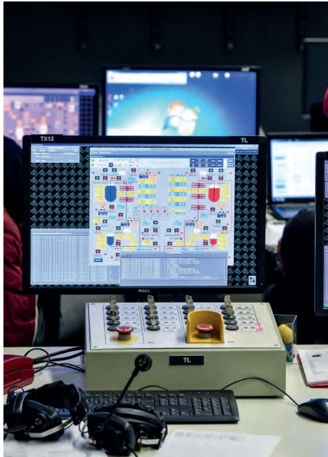
The test director's station: The test is followed through computer screens and can be interrupted in the event of an emergency.
