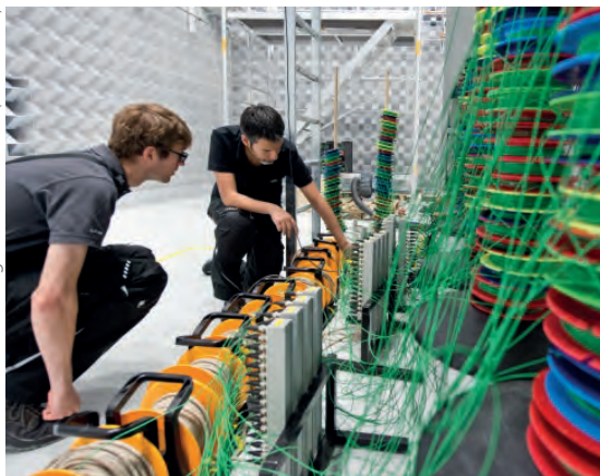
The cable routing for 200 sensors must be organised in such a way that faults and defects can be remedied as quickly as possible
