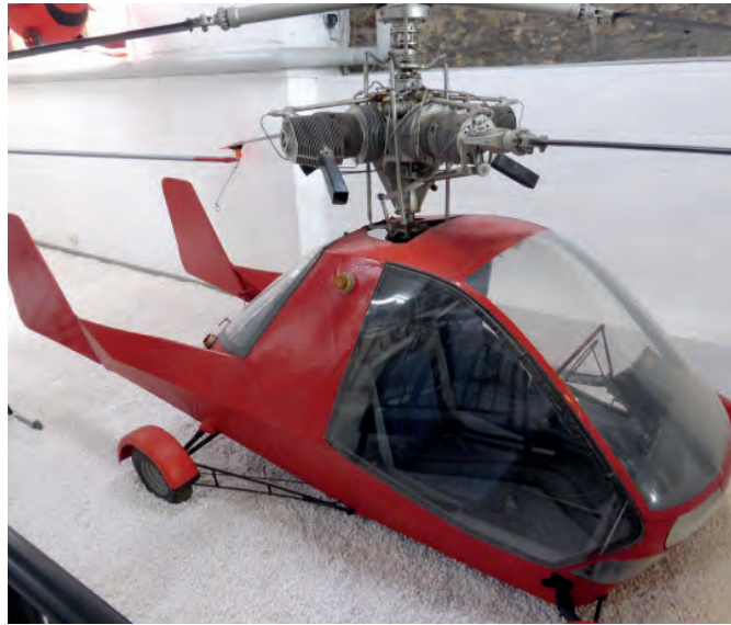
The Wagner Rotocar from 1960 was intended to combine helicopter and motor vehicle systems. The two rotors were powered by a three-cylinder radial engine.
