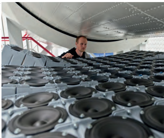
The loudspeaker array used for projecting sound fields onto the demonstrator. It has 132 elements and can be moved to almost any position on the surface.
