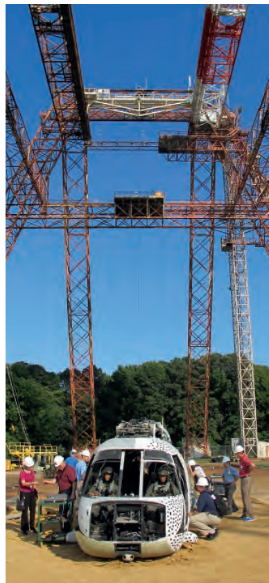
Scientists study the helicopter fuselage after the impact Right: sequence from the TRACT2 crash test
