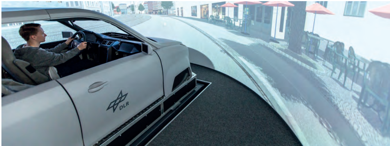
In a so-called modular mock-up, the test driver tests new assistance and automation systems, combined with new vehicle concepts, and has a complete panoramic view.
