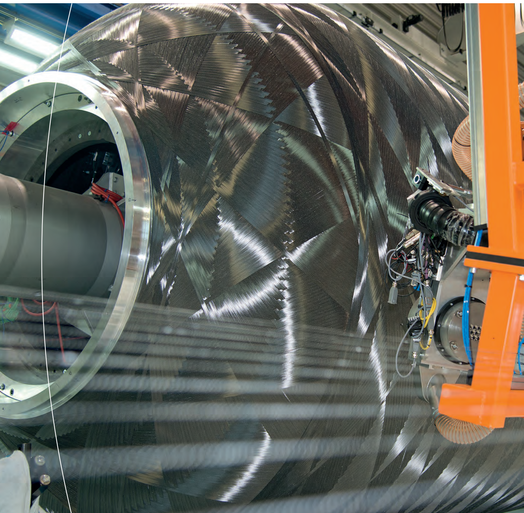
The unique facility in the Center for Lightweight Production (Zentrum für Leichtbauproduktionstechnologie; ZLP) in Augsburg combines two production processes into one: when producing rocket boosters made of CFRP, rovings can be wound onto the core (see image) and wider tapes can be laid.
