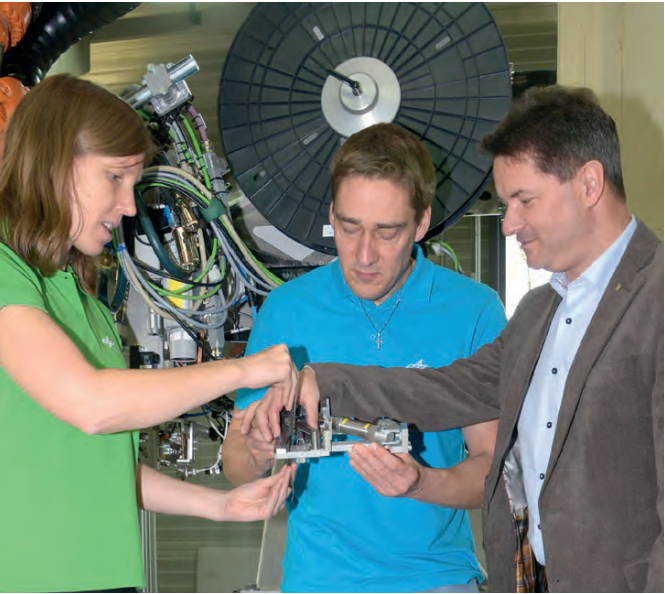
Kupke (right) in conversation with Mona Eckardt and Roland Glück. The carbon fibres are cut with the help of a blade (centre of image) – one of the many technical challenges in automated booster production.
