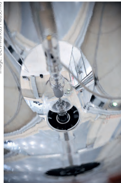
All lamps are equipped with a mirrored aluminium reflector and can be focused individually onto the samples
