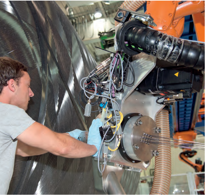
A robot winds the dry fibres onto the pressure vessel. In the development phase, people still check that the process is running smoothly.
