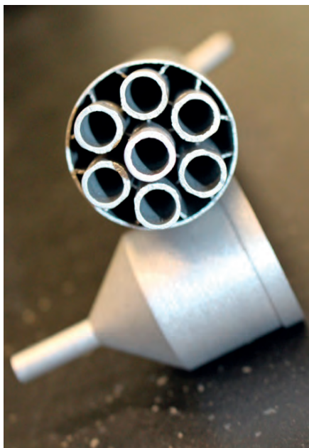
The small tubes inside the cold start module contain the metal hydride. The heat transfer fluid flows around them.
