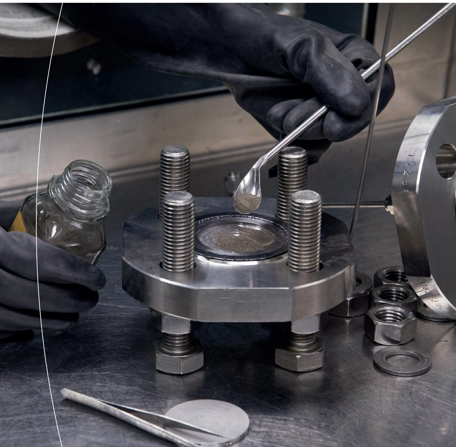
The metal hydride powder is put into an experimental set-up. The scientists work in a so-called glovebox that shuts out oxygen.
