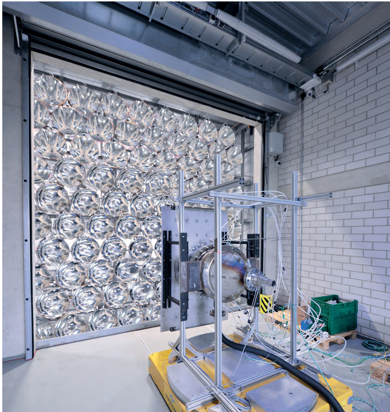
An equivalent power of 10,000 times the solar radiation focused on one spot: 149 Xenon spotlights can be concentrated on a 20 by 20 centimetre area. This results in temperatures of up to 3000 degrees Celsius.
