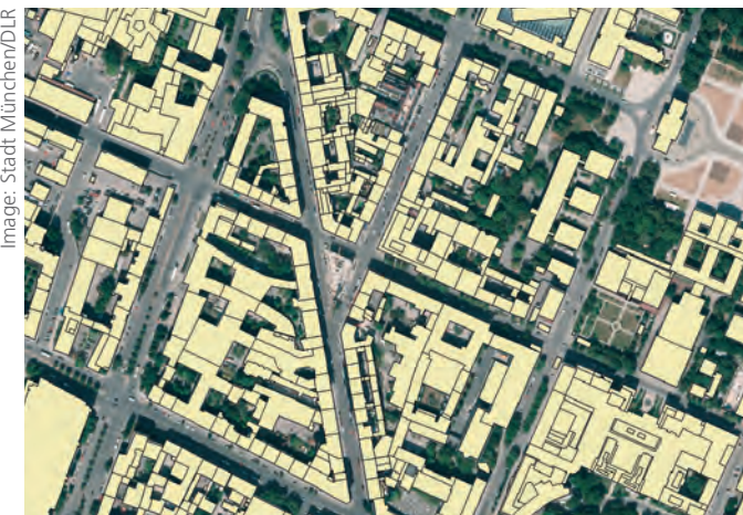
With the aid of cadastral data, house outlines can be filtered out of aerial photographs. Roof surfaces are thus clearly recognisable.
