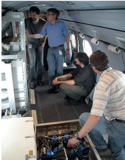
Preparation for a test flight with the Franco-German climate mission MERLIN (Methane Remote Sensing Lidar Mission) on board HALO. CHARM-F will be tested on the flight. CHARM-F (CH4 Airborne Remote Monitoring) is an aircraft-borne integrated path differential absorption (IPDA) lidar. It can be used to quantify gradients of concentration as well as carbon dioxide and methane land-atmosphere fluxes, both from anthropogenic point sources and from broader natural sources
