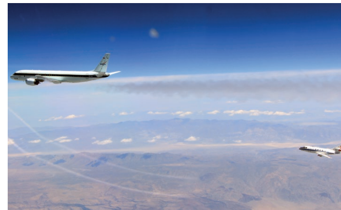
Environmentally-friendly flight: Joint DLR / NASA research flights have shown that adding biofuel to kerosene reduces aircraft soot particle emissions by more than 50 percent compared to conventional fuel. Scientists on board the DLR Falcon measured the composition of the exhaust gas from a DC-8 that is flying in front of them.
