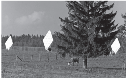
1971 VHF interferometer for measuring satellite orbits
