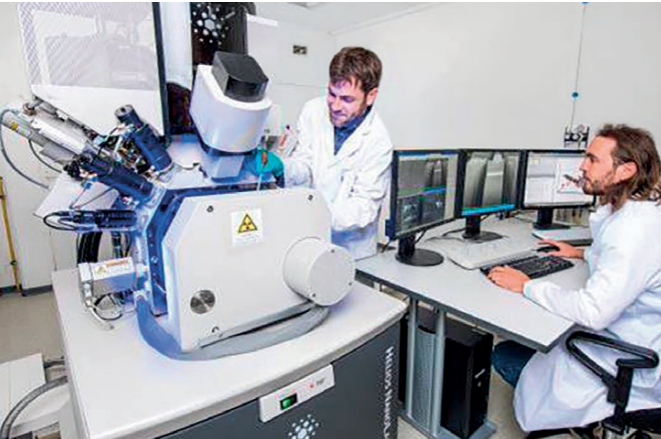
Philipp Watermeyer (left) and Mario Eggeler with the dual beam focused ion beam system. Material samples can be cut into very thin slices using this system. An image of the surface of each of the slices is made using an electron microscope. A digital 3D image-like dataset of the material is then calculated from the individual slices with a computer.
