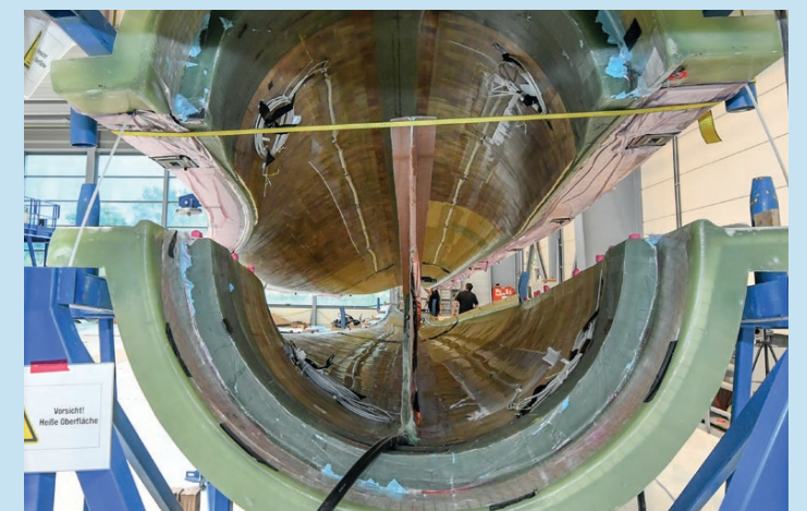
After the two halves are put together to see how they fit and adjusted precisely, they are welded and cured.
