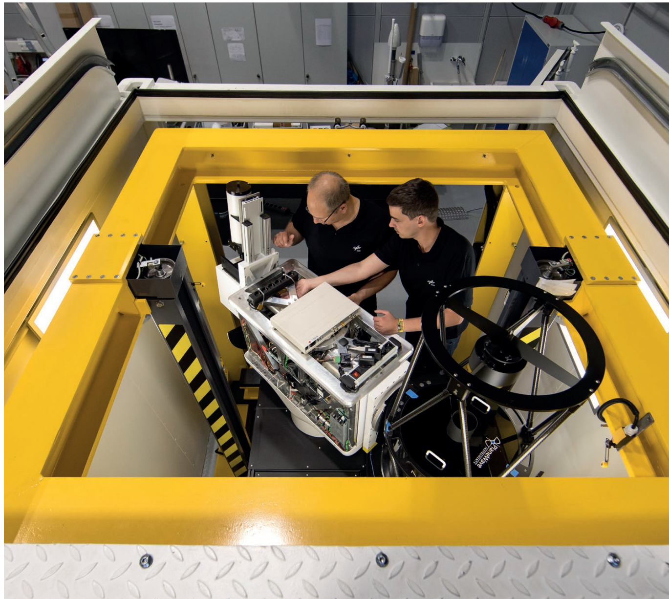
The special feature of the mobile space debris observatory is the lifting platform for the telescope. It is extended upwards through a sunroof.
