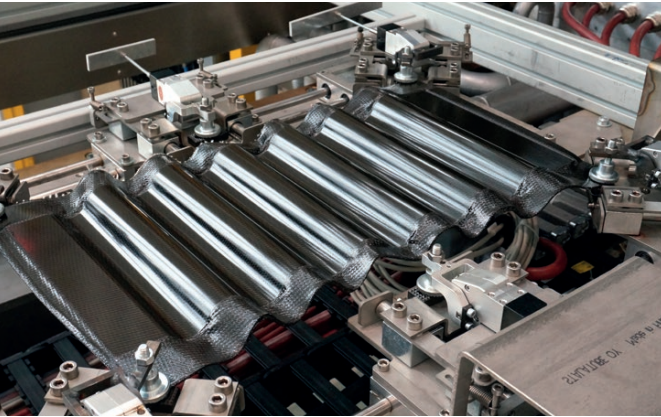
Component in tenting frame after thermoforming (hot pressing)
