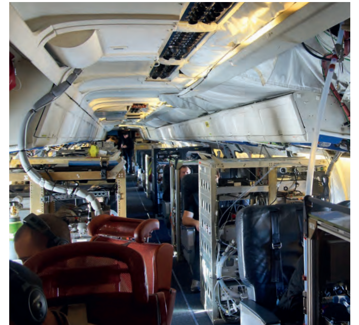
In the cabin of the DC-8: The hoses, where the outside air is led into the numerous instrument racks, are clearly visible. Approximately half of the instruments on board come from DLR.
