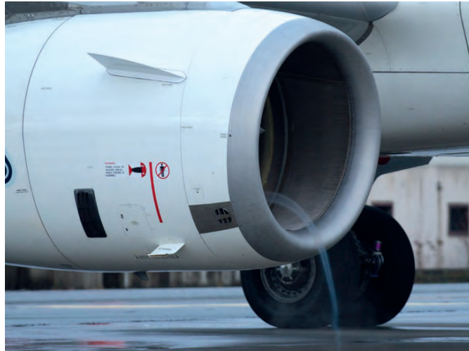
During the ground measurements, light blue-grey exhaust air vortex can be seen, which 'falls' from the engine of the A320 ATRA.
