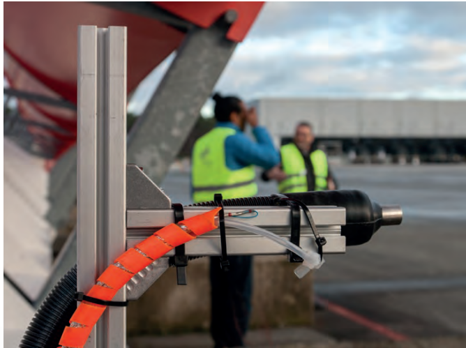
The exhaust gases are directed to the measuring instruments via an air inlet and a hose system
