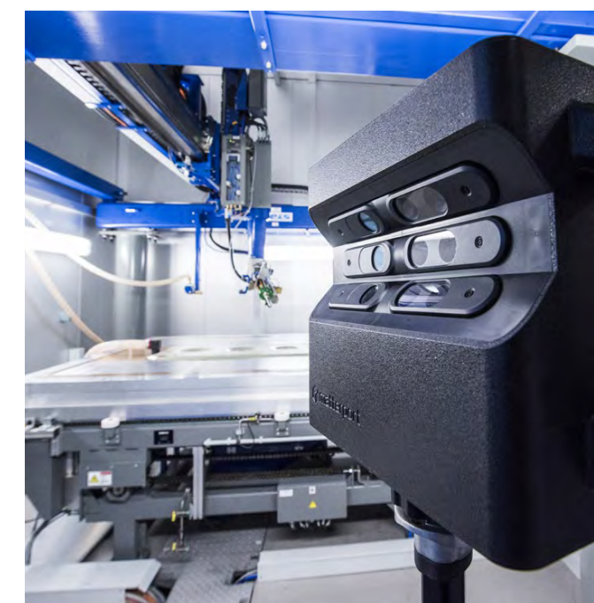
Street View' for indoors – a 3D scanner on the production line at DLR Stade.
