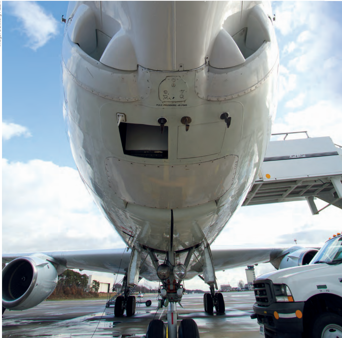
Recognisable in the fuselage of NASA's DC-8 – air inlets for exhaust gas measurements.
