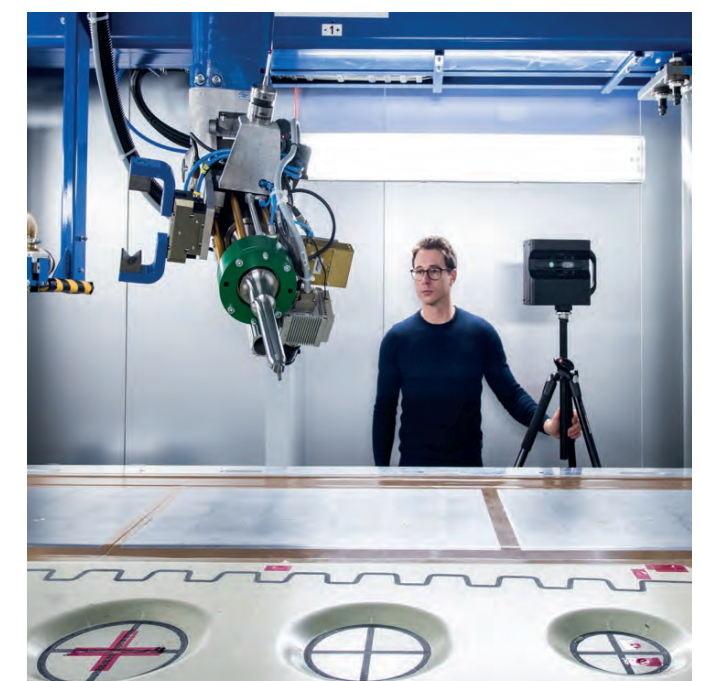
Birth of a digital twin – the camera scans every corner and every angle of the component.
