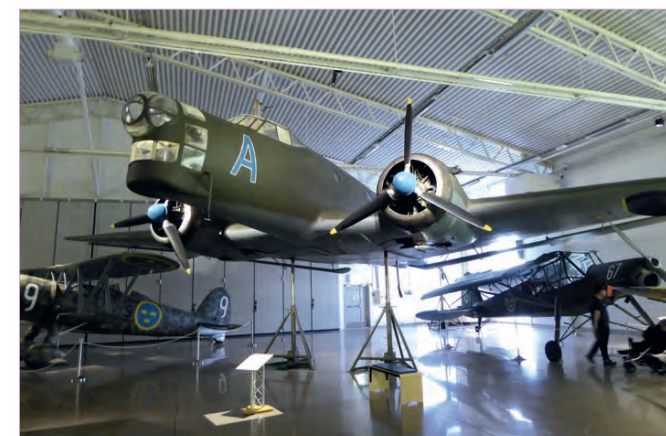
With this medium-range bomber, Junkers left the traditional corrugated iron construction in favour of an aerodynamically improved smooth skin planking. The exhibited specimen is the world's only remaining Junkers Ju 86.
