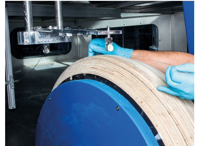
System for winding fibre-reinforced oxide ceramics at the DLR site in Cologne
