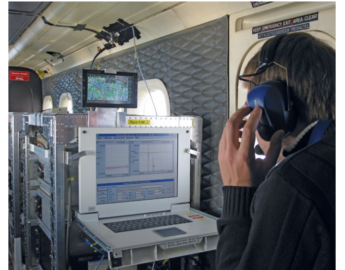
The Channel Sounder in DLR's Dornier Do 228-101 (D-CODE) research aircraft
