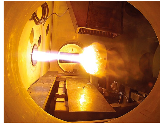
A re-entry capsule made of fibre-reinforced oxide ceramic undergoing testing in a plasma tunnel
