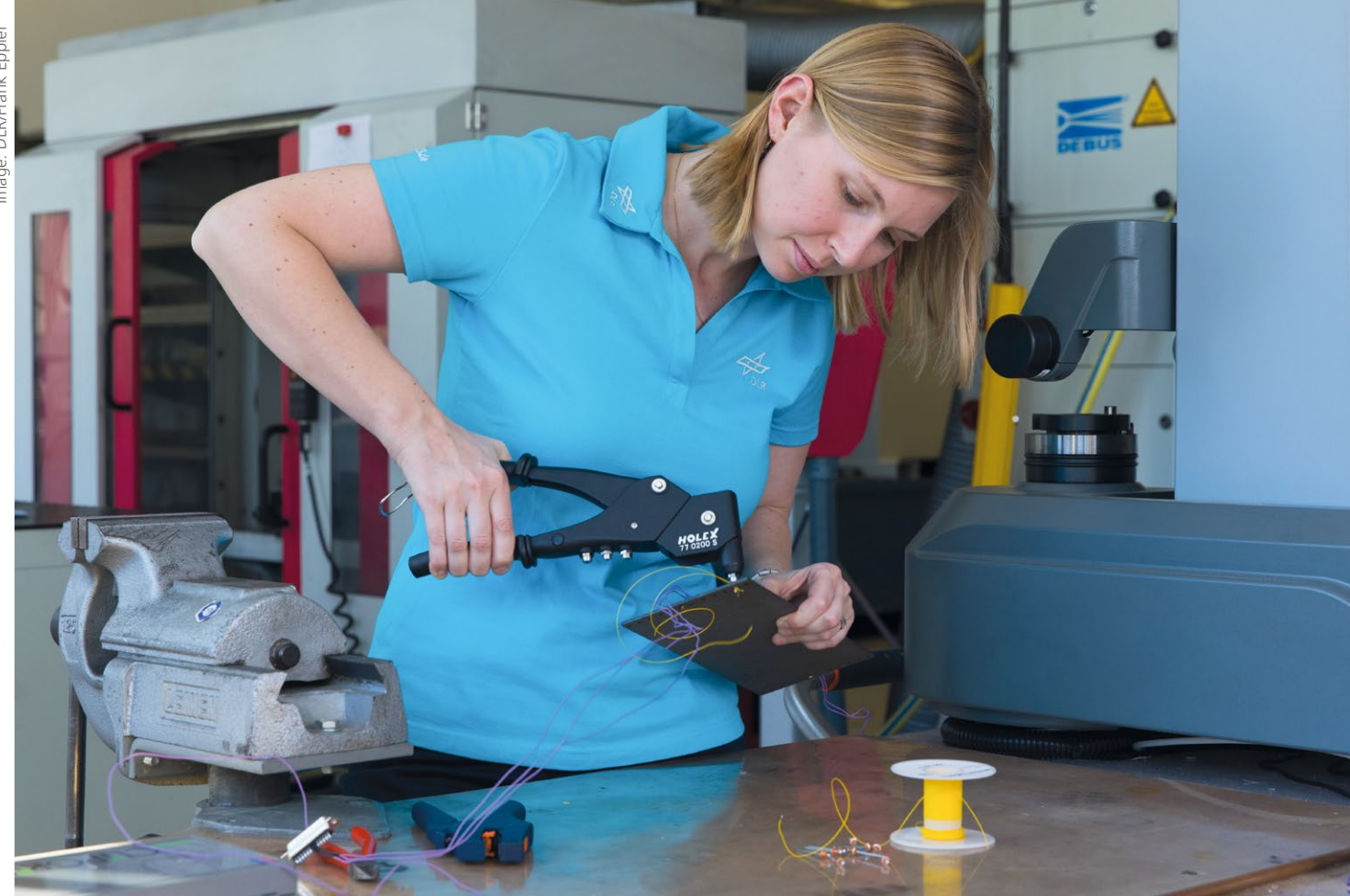
Tina Stäbler in the workshop of the Institute of Structures Design in Stuttgart: The attachment of contacts on the sample plate is based on a carefully considered system. The network of measuring paths should be as precise as possible.
