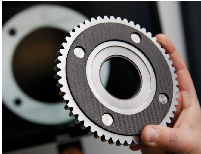
Propeller brake disc for the Airbus 400 M; the friction lining is made of black fibre-reinforced ceramic.
