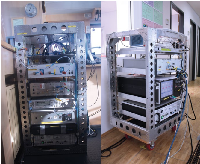
The Channel Sounder in operation – transmitter (left) and receiver unit (right).
