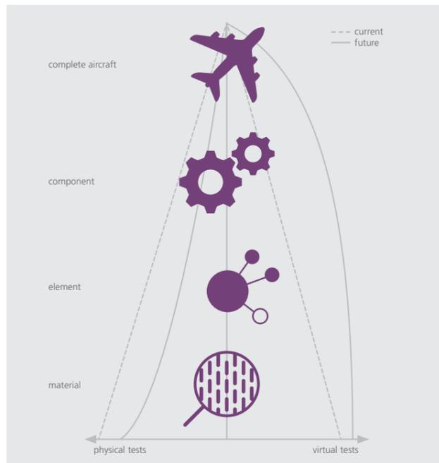
This test pyramid from the aeronautics sector shows the development steps from initial material tests to the design and testing of individual elements and components and then on to the complete aircraft system. In future, physical verification of certifications will be increasingly supplemented by virtual tests, and perhaps even replaced by them in the longer term.
