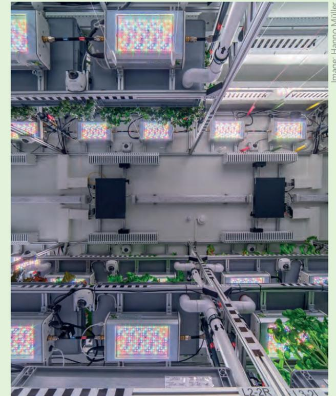
View of the water-cooled LED systems from below. These shine light on the plants in a precisely coordinated day-night rhythm.
