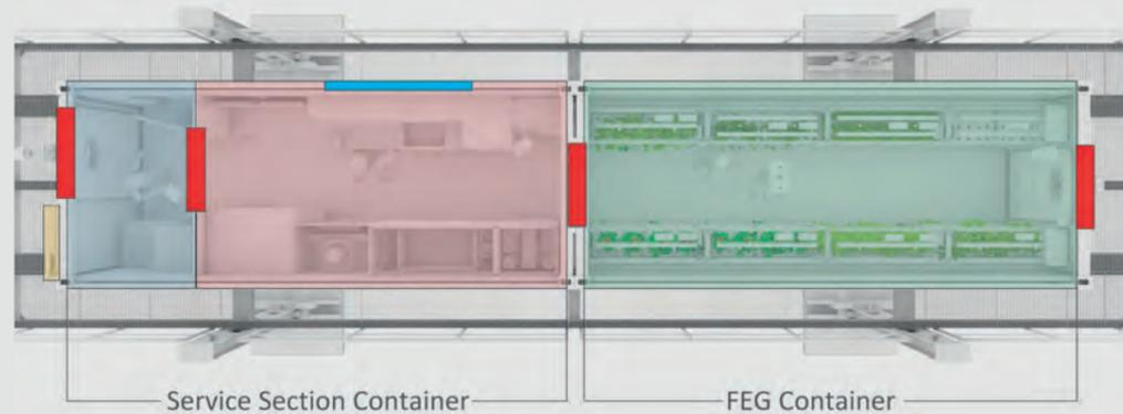
The EDEN ISS Service Section container houses an airlock (shown in blue) for changing Antarctic clothing. Next to it (red) is the area for the atmosphere management system, the nutrient supply system, the thermal regulation system and the data handling system. The Future Exploration Greenhouse (green) container generates fresh produce in 12.5 square metres.
