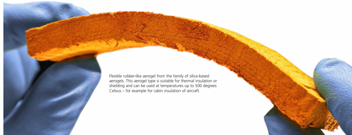
Flexible rubber-like aerogel from the family of silica-based aerogels. This aerogel type is suitable for thermal insulation or shielding and can be used at temperatures up to 500 degrees Celsius – for example for cabin insulation of aircraft.
