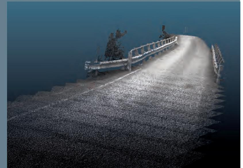
Three-dimensional model of a bridge, also based on a point cloud generated by IPS.
