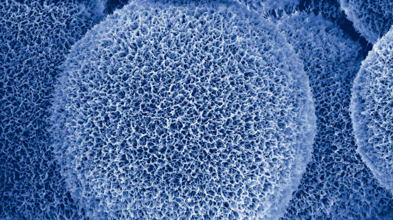
A new biopolymer aerogel developed by DLR scientists in a laboratory experiment. The spherical and filamentary structures are created when chitosan is combined with a thermoset.
