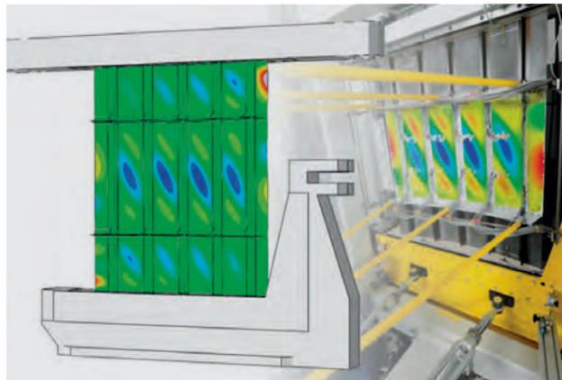
Materials testing at the buckling point – performed here on both virtual and physical test benches.
