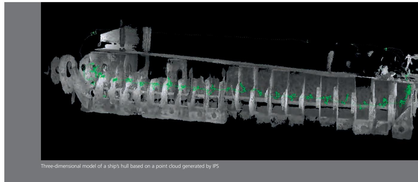
Three-dimensional model of a ship's hull based on a point cloud generated by IPS
