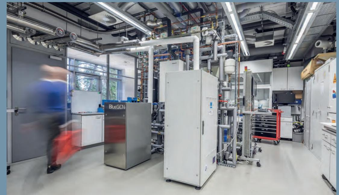
"Storing heat is much cheaper than storing electricity," stresses Carsten Agert. Against this backdrop, DLR is conducting research into electricity-based heating systems combined with thermal storage at its Combined Heat and Power (CHP) Laboratory. If the heat is generated at a time when there is a surplus of electricity, this makes the energy system more flexible.
