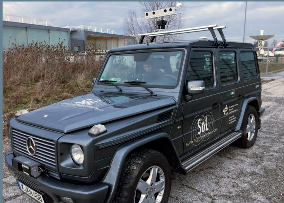
IPS is also used for research in the areas of autonomous driving and surveying of road infrastructure, as shown here with a research vehicle from the DLR Institute of Communications and Navigation.
